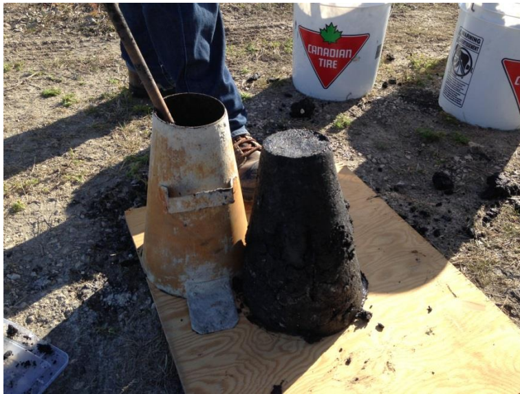
Photo 5. Slump testing the lagoon solids.
