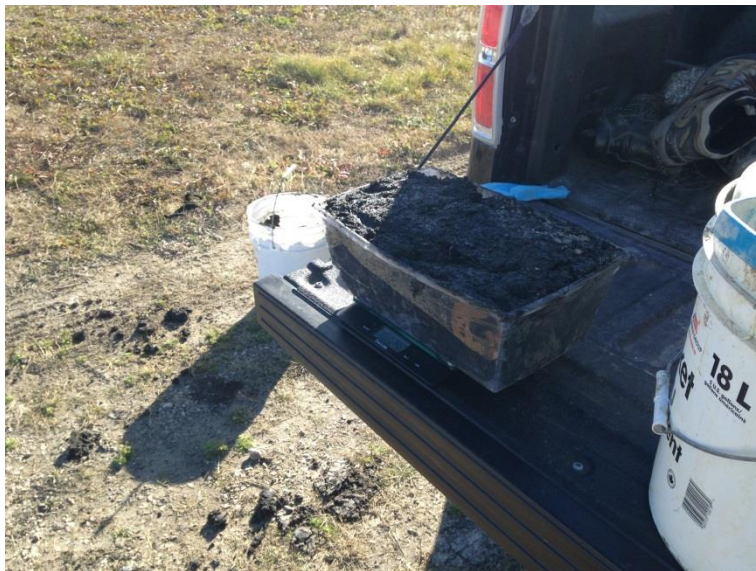
Photo 6. Density testing the lagoon solids.
