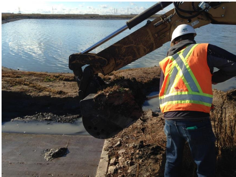
Photo 4. Shovelling solids from back hoe into sampling pail.
