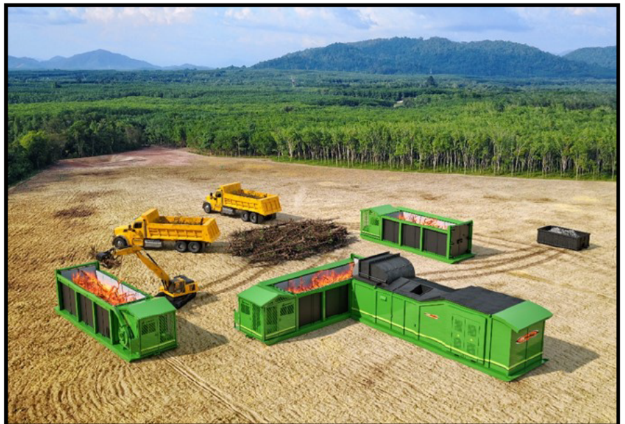
One Power Module Powering Three Air Curtain Machines and making Biochar
