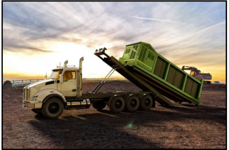
Roll-Off FireBox Being Delivered
