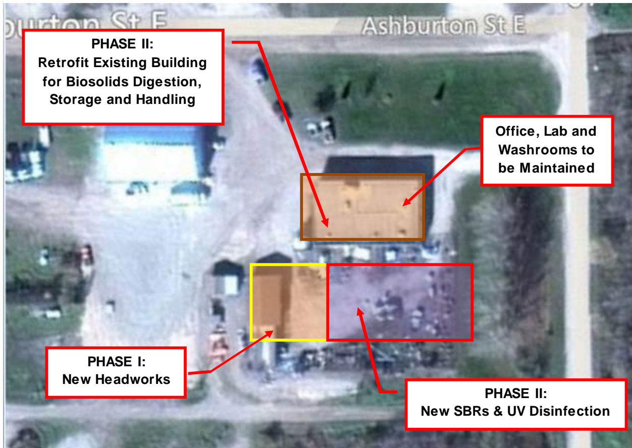
Plate 2-2: Phase I and Phase II works for the Viriden WWTF Upgrade Project.
