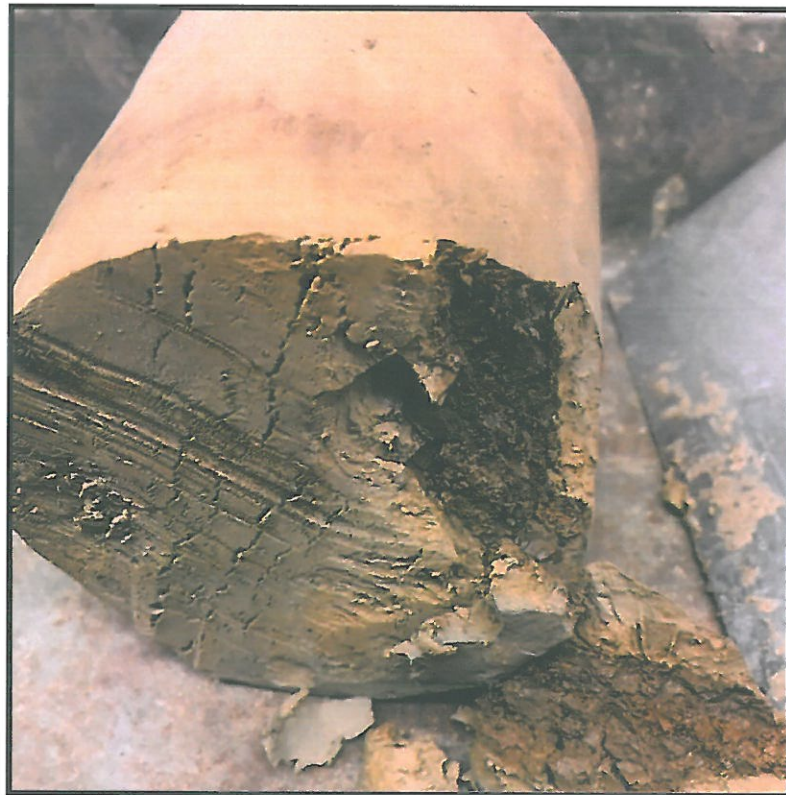
PHOTOGRAPH #4: Sample ST6 after breaking apart.
