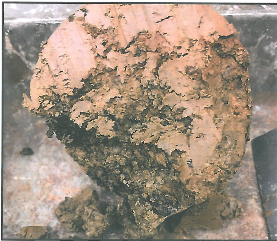
PHOTOGRAPH #2: Sample ST4 after breaking apart.
