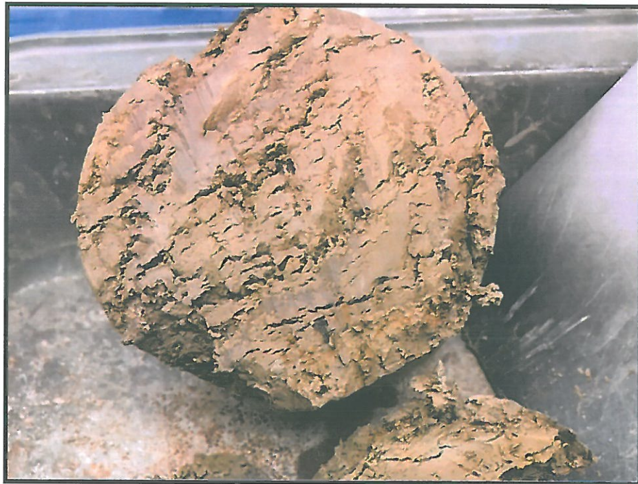
PHOTOGRAPH #6: Sample ST7 after breaking apart.
