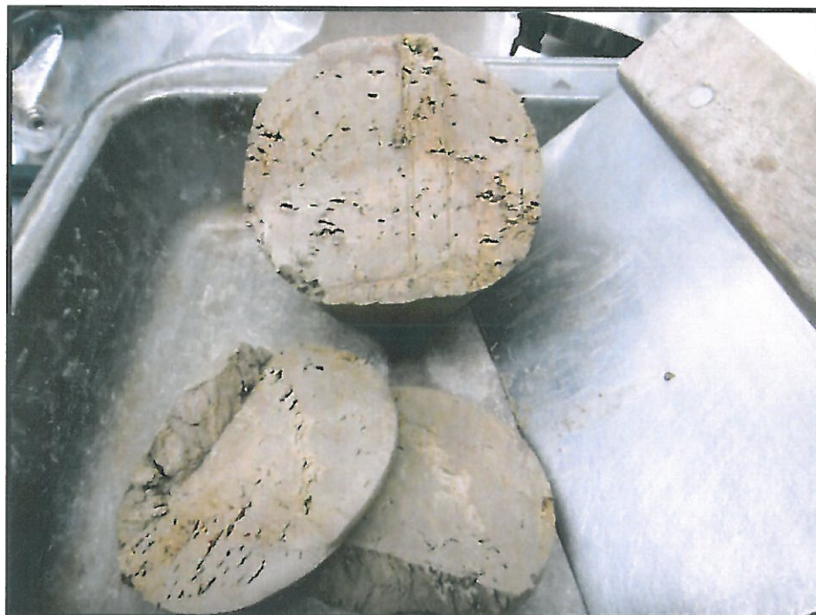
PHOTOGRAPH #2: Sample ST2-A after breaking apart.
