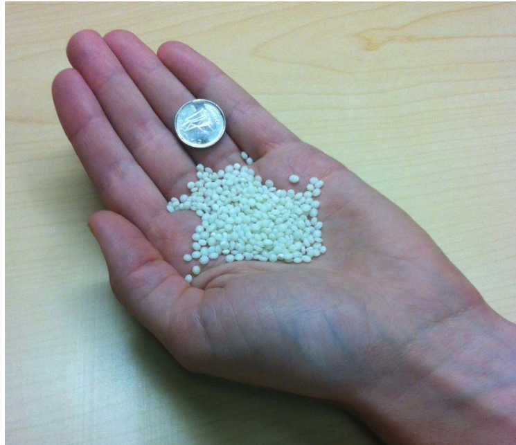
Figure 4 Struvite harvested from a wastewater treatment plant
