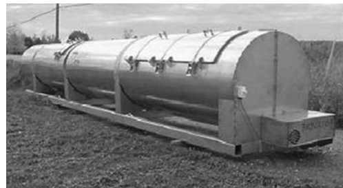
In-vessel composting system
